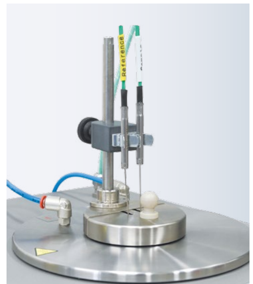
DTA 552-Ex – detail of the furnace
